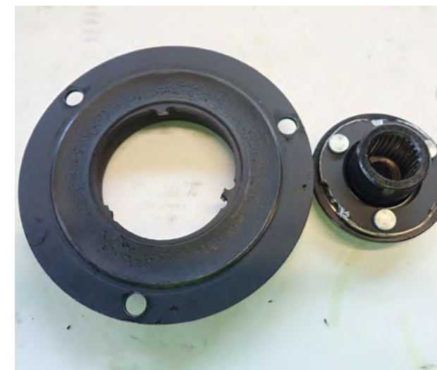
Fig. 1 Protection anti-surcharge cassée
